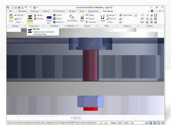
Create and modify multiple screw connections complete with drilled holes and accessories (such as nuts and washers) in one step.
