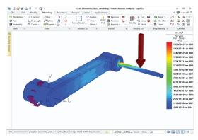
Easily detect weaknesses in your design before performing expensive tests on physical prototypes.
