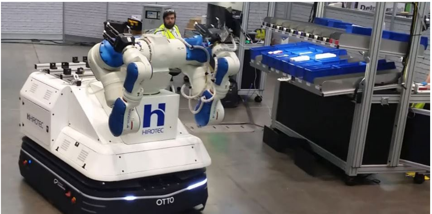
FIGURE 2 – HIROTEC Robot Transferring Materials Between Work Cells in the X-Factory at LiveWorx 2018
